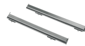
GT1P-2 Partially extractable telescopic guides (1 level) for ovens with metal frames. Length: 355.5 mm, extraction: 285 mm. Material: Stainless steel AISI 430 polished.
