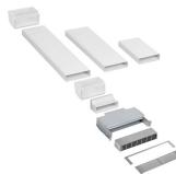
Recirculating kit for Hobd: tubes + regenerable anti-odor filter + grid in stainless steel with magnetics fix (easy to remove) that fit in a plinth of min. 6 cm. The ceramic filter can be regenerate up to 10 times by putting it inside the oven at 250° for 1 hour.
