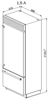
Voltage (V) 220-240 V Frequency (Hz) 50 Hz Power supply cable 250 cm length
