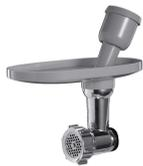
Alluminum alloy body, ferrule and cochlea. Included accessories: 3 stainless steel discs for mincing (coarse Ø 8 mm, medium Ø 4,2 mm, fine Ø 3 mm), plastic Sausages and Kebbe accessory, a silicon disc for cleaning and a pestle to introduce better the ingredients.
