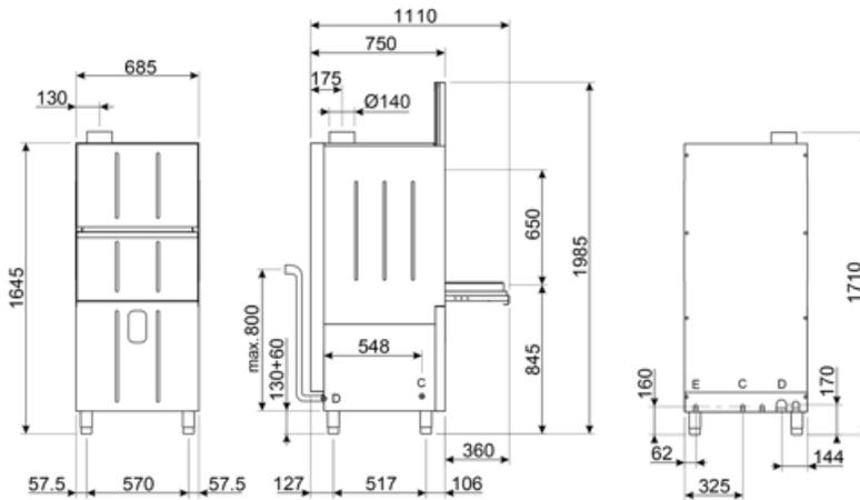
D = SCARICO 1 1/2", VIDANGE 1 1/2", DRAIN 1 1/2", ABFLUSS 1 1/2", DESAGÉE 1 1/2", CИВВ 1 1/2"
