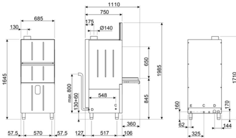
D = SCARICO 1 1/2", VIDANGE 1 1/2", DRAIN 1 1/2", ABFLUSS 1 1/2", DESAGŪE 1 1/2", CIBB 1 1/2"
