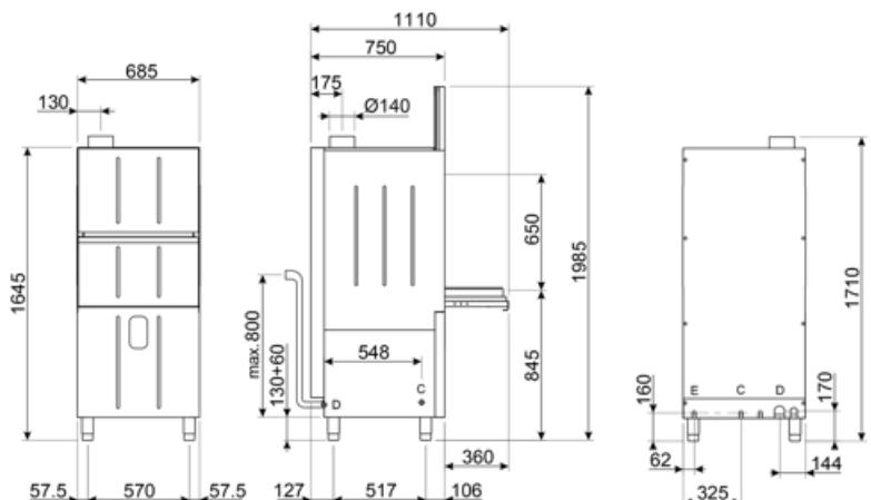
D = SCARICO 1 1/2", VIDANGE 1 1/2", DRAIN 1 1/2", ABFLUSS 1 1/2", DESAGÜE 1 1/2", CIBB 1 1/2"
