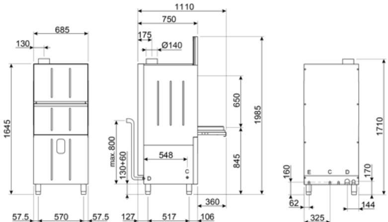
D = SCARICO 1 1/2", VIDANGE 1 1/2", ABFLUSS 1 1/2", DENAGÜE 1 1/2", CBIB 1 1/2"
