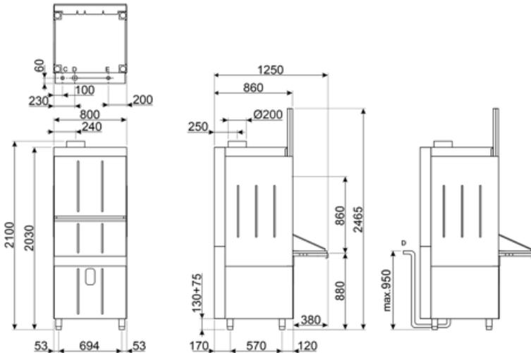
D = SCARICO 1/2", VIDANGE 1/2", DRAIN 1/2", ABFLUSS 1/2", DÉGÂGE 1/2", CIBB 1/2"
